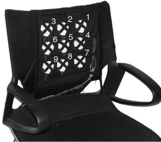
Figure 1. The haptic back display. Shown here is a 3-by-3 factor array. Each factor is fastened, by two crisscross elastic bands, to a piece of supporting fabric that is draped over the back rest of an office chair.
