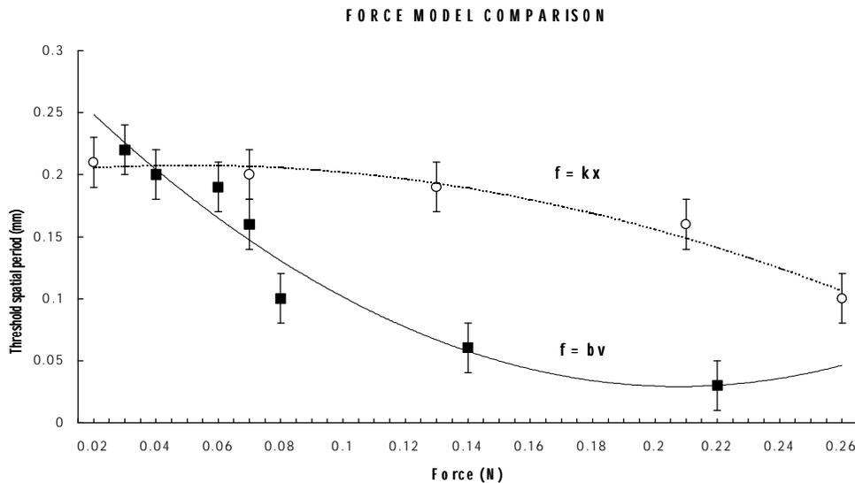
Figure 7. Threshold spatial period as a function of total force for stiffness ( $f=kx$ ) and damping ( $f=bv$ ) force models on the PHANToM.
