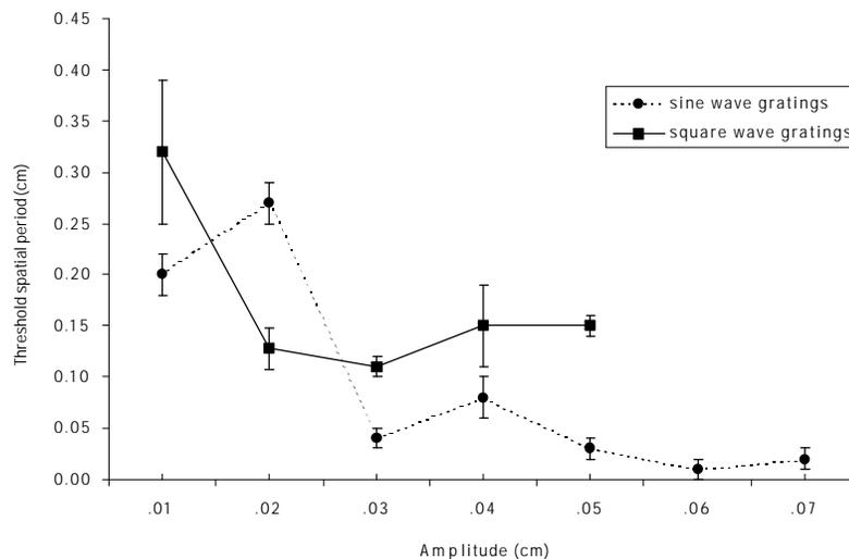
Figure 5. Sine and square wave grating resolution for the 3-DOF device.
