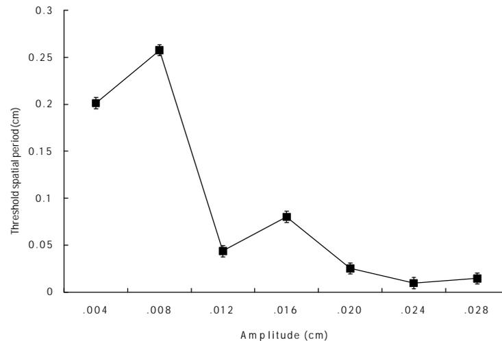
Figure 3. Threshold spatial period in cm as a function of grating amplitude for the 3-DOF device.
